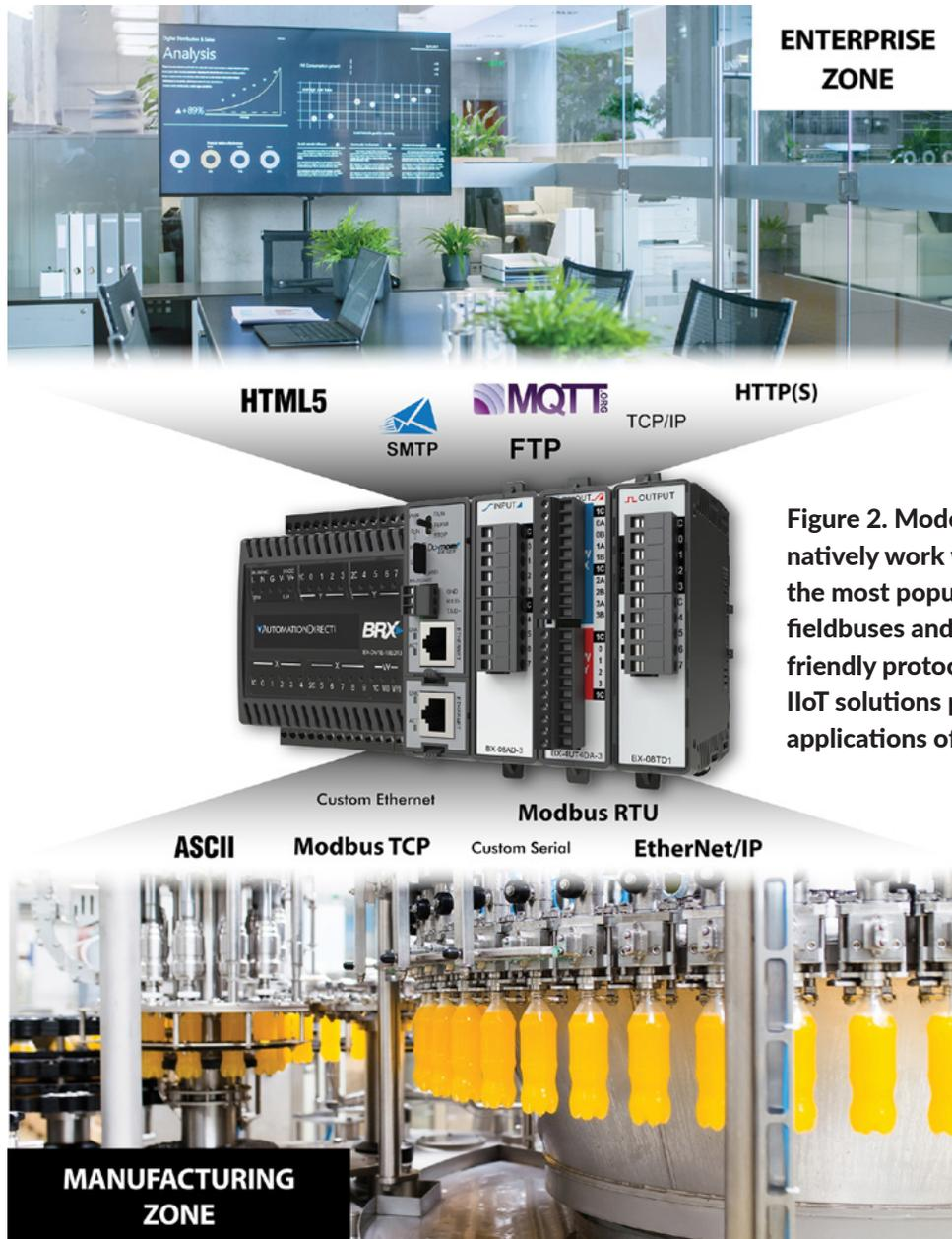
Figure 2. Modern PLCs natively work with the most popular OT fieldbuses and multiple IT-friendly protocols to make IIoT solutions practical for applications of all sizes.
