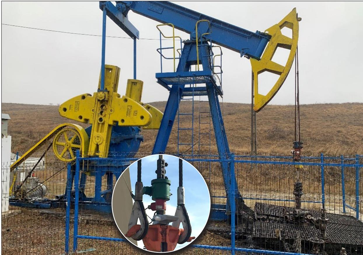
Figure 2. Data is collected from load accelerometers installed on the pumpjack donkey arm to monitor oil well efficiency and detect issues that could result in oil well collapse. Inset: The pumpjack donkey arm lift.
