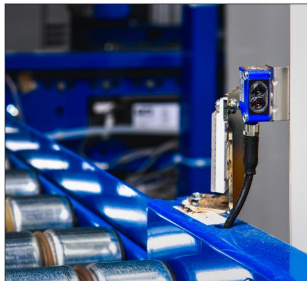
Figure 3. Photoelectric sensors are especially suitable for detecting the presence or absence of larger targets, such as conveyed boxes.
