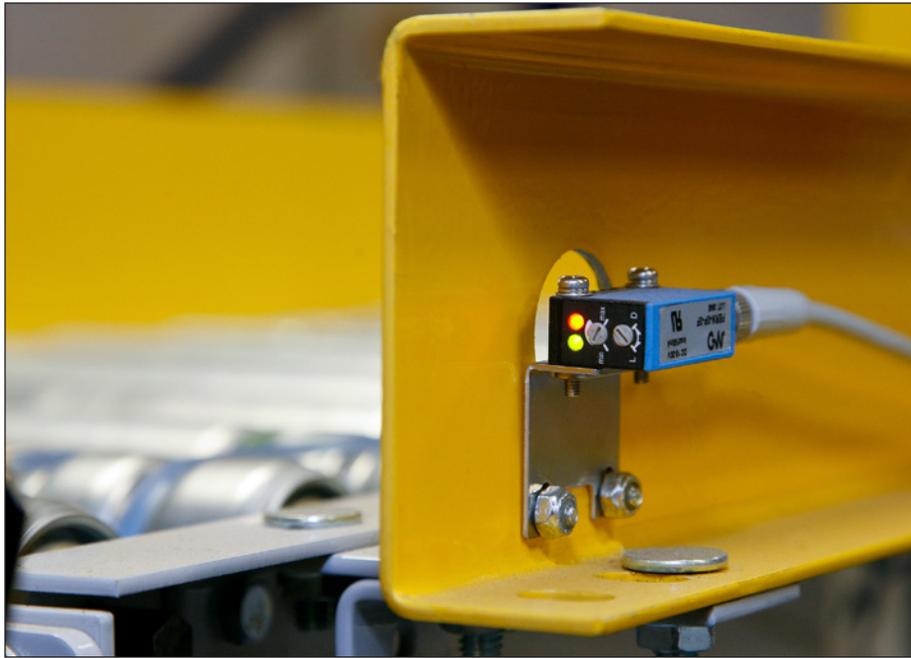
**Figure 1.** Many discrete sensors are available with IO-Link, so they can provide advanced data and connectivity, going far beyond basic on/off signals, with simplified field installation.
