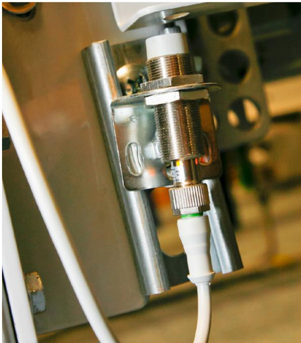
Figure 2. Proximity sensors using capacitive, magnetic, or inductive technologies are a compact way of detecting various targets.
